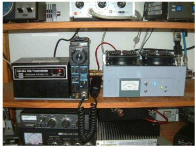
Most 23cm stations run from a few mW up to ~ 15 watts. This may be from a standalone transverter, with an optional amplifier module, or an elderly MMT1296, and in some cases a transceiver with 1296 MHz included. The availability of surplus amplifiers and amplifier kits, recently, have allowed many to run higher power than before.
